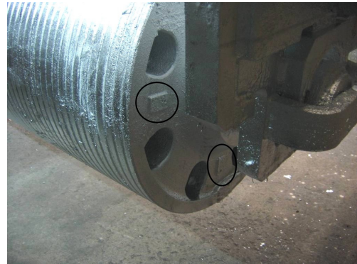
Fig.2. The circled areas show the testing samples which were welded on a sink roll.
